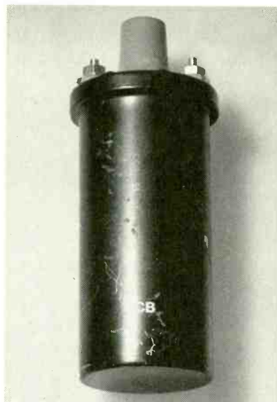
FIG. 5—VIRTUALLY ANY automobile ignition coil can be used for T1.
